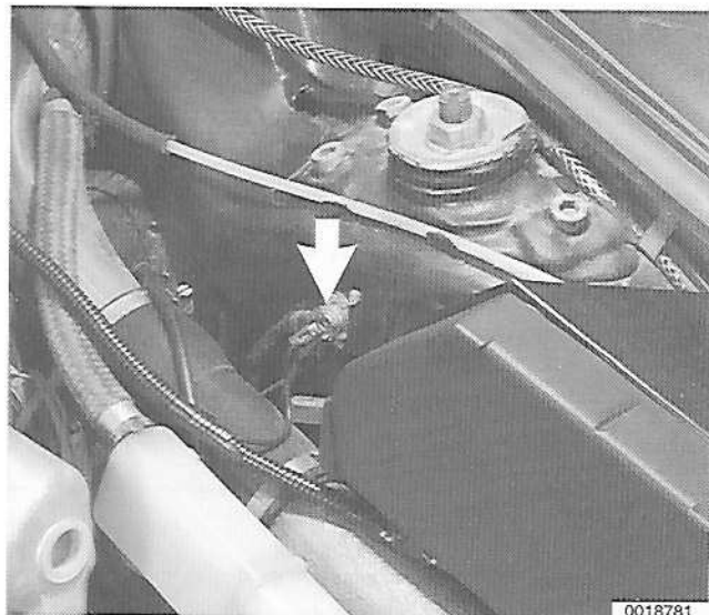
⚡ Battery ground location G104 (arrow).
